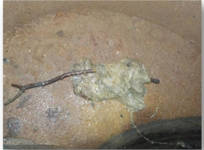
Stick Blocking Outlet Pipe Resulting in Ragging
