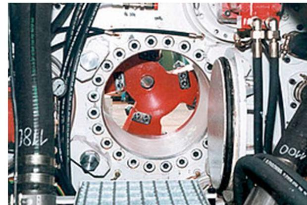
Access Door for Worn Cutter Replacement
