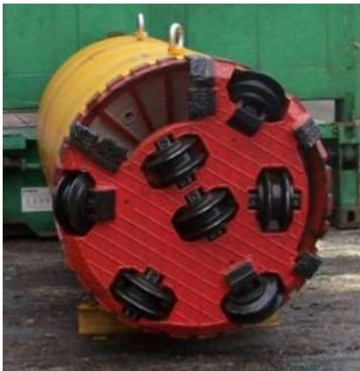
Slurry MTBM with Rock Cutter Head
