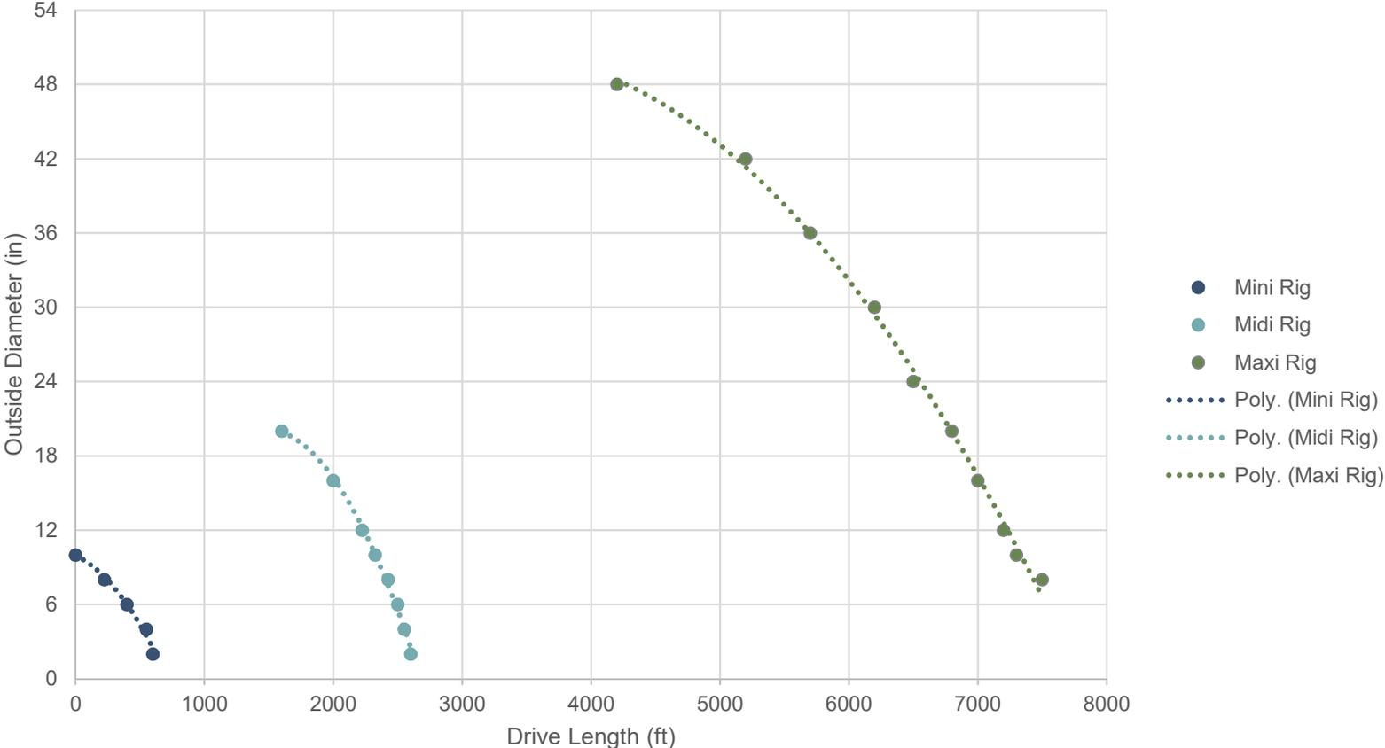
HDD Drive Length Capabilities – some max lengths require steel pipe
