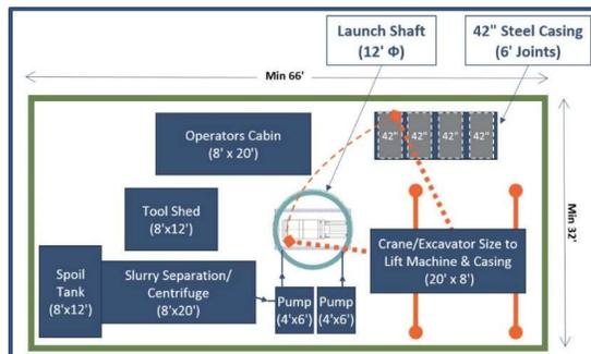
**42" Two-Pass MTBM Installation**
