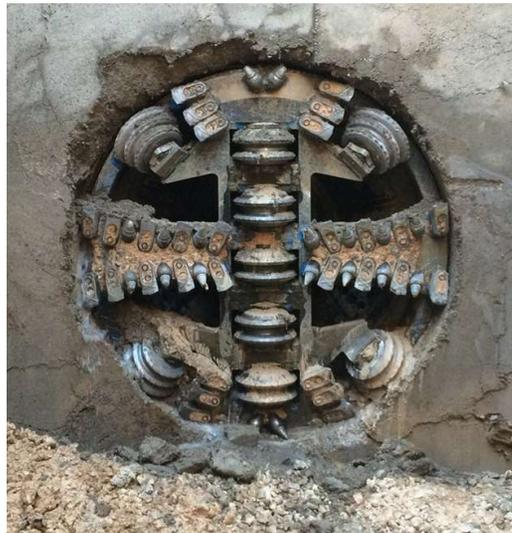
Slurry MTBM with Mixed Face Cutter Head
