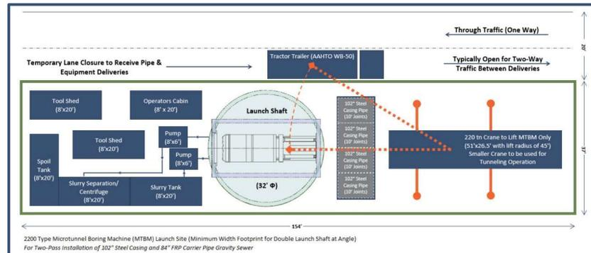
2200 Type Microtunnel Boring Machine (MTBM) Launch Site (Minimum Width Footprint for Double Launch Shaft at Angle)
