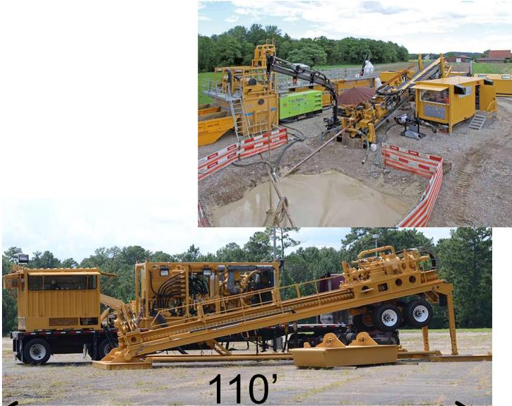
Large HDD Drill Rig
